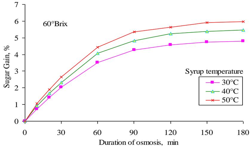
Fig.5 Sugar with duration of osmosis at 60°Brix syrup concentration at three different syrup temperatures.
