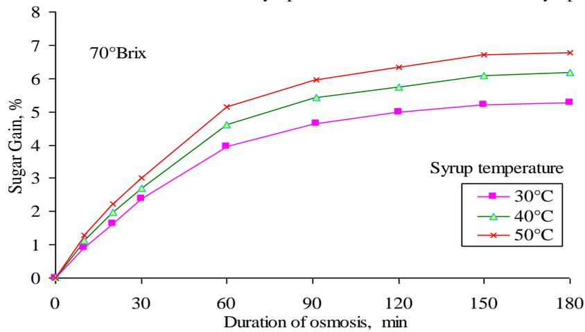
Fig. 6 Sugar gain with duration of osmosis at 70°Brix syrup concentration at three different syrup temperatures.
