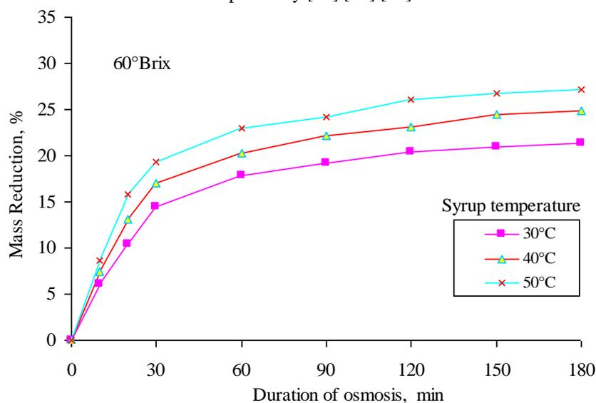
Fig.8 Mass reduction with duration of osmosis at 60°Brix syrup concentration at three different syrup temperatures.
