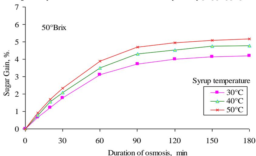
Fig. 4 Sugar gain with duration of osmosis at 50°Brix syrup concentration at three different syrup temperatures.
