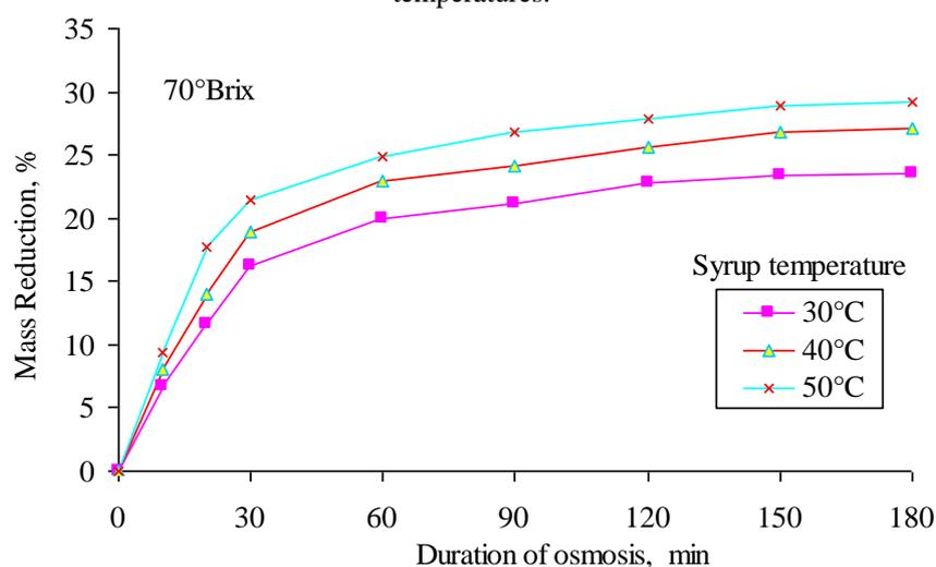
Fig.9 Mass reduction with duration of osmosis at 70°Brix syrup concentration at three different syrup temperatures.
