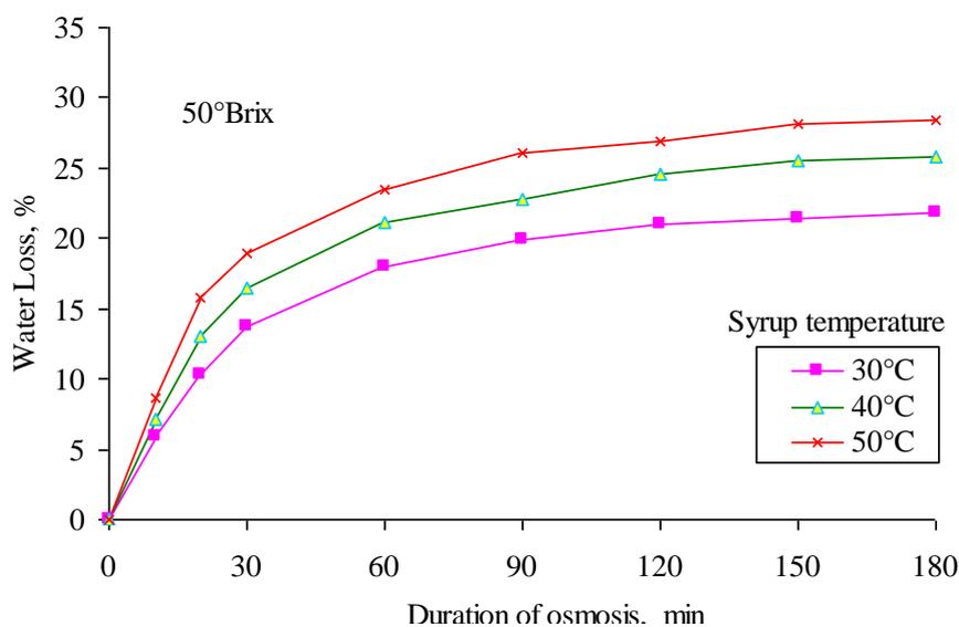
Fig. 1 Variation in water loss with duration of osmosis at 50°Brix syrup concentration at three different syrup temperatures
