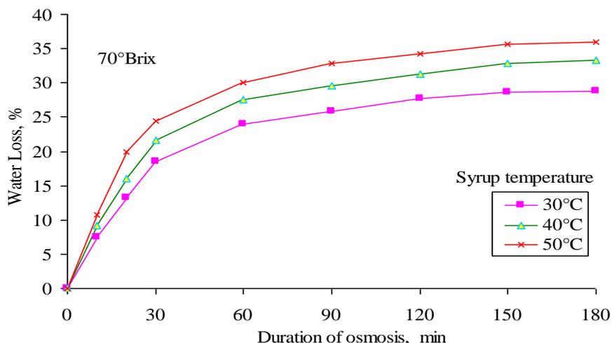
Fig. 3 Water loss with duration of osmosis at 70°Brix syrup concentration at three different syrup temperatures
